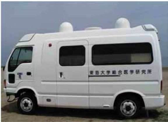
Fig. 5 Prototype super ambulance Two diversity antenna mounted on the roof
